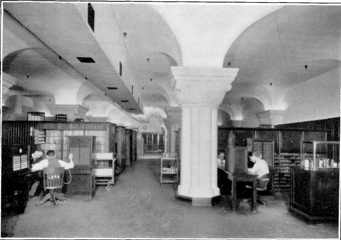
Dry Cell Testing Laboratory of the National Carbon Company—Each year about 100,000 dry cells are tested, requiring an average of 7,000 readings a day. The laboratory is kept at a constant temperature of 70° F. at 55% humidity. A large proportion of the readings are made with the aid of telephone switchboards
